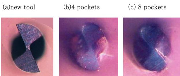
Fig.3 Change of bottom cutting edges(φ 0.2mm)
