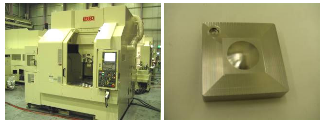
Fig.3 Developed MC with on-machine measurement system(left) Sphere shaped model used for measuring test(right)
