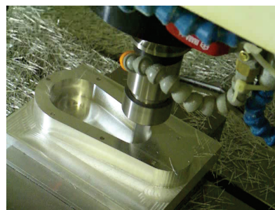
Fig.4 Outlook of end milling Mg-alloy parts
