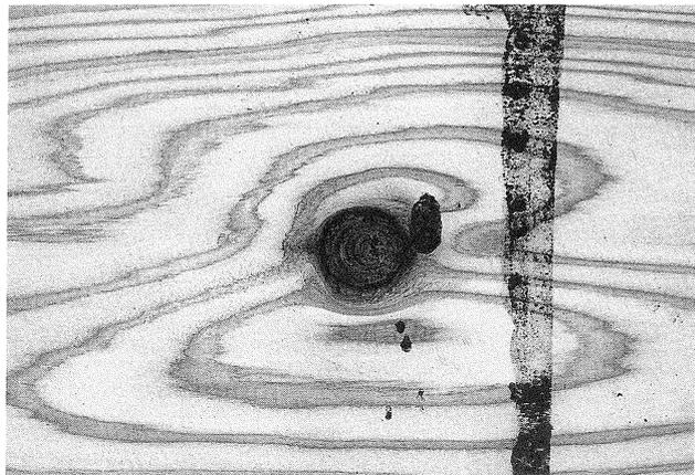
Fig.3 A Case of Dead Knot Located on Center of The Timber
